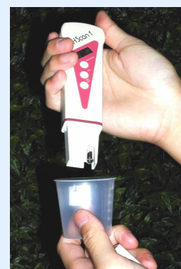
A hand held pH meter for measuring the acidity of water.
